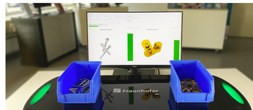
Using inductive near-field positioning, IndLoc® recognizes fill level and materials.
